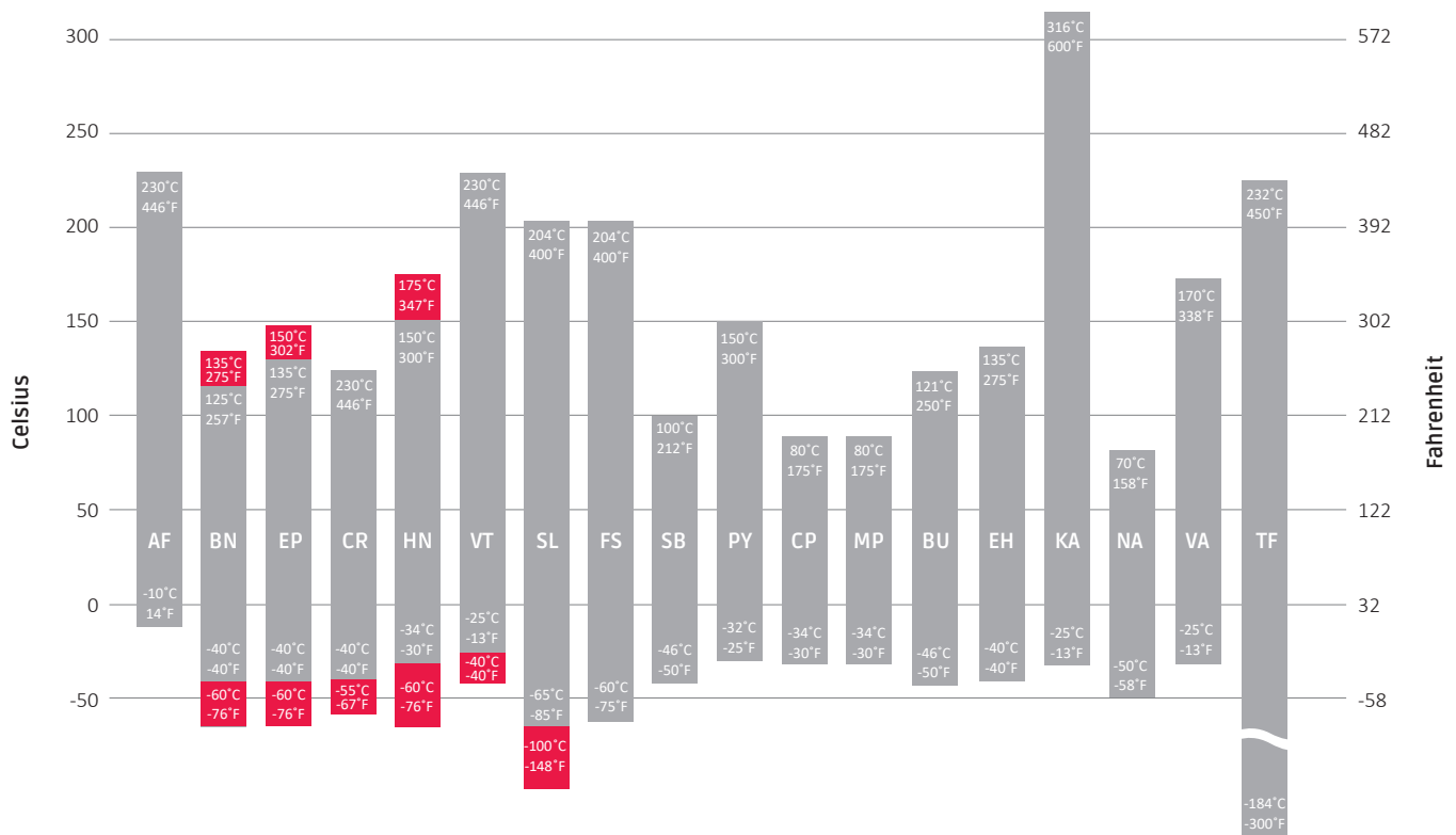
Illustration 5.4, Typical O-Ring Material Working Temperature Ranges
