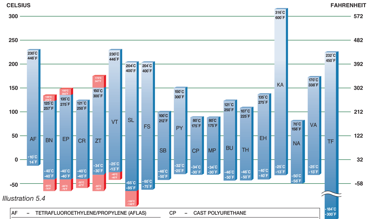
Typical O-ring Material Working Temperature Ranges
