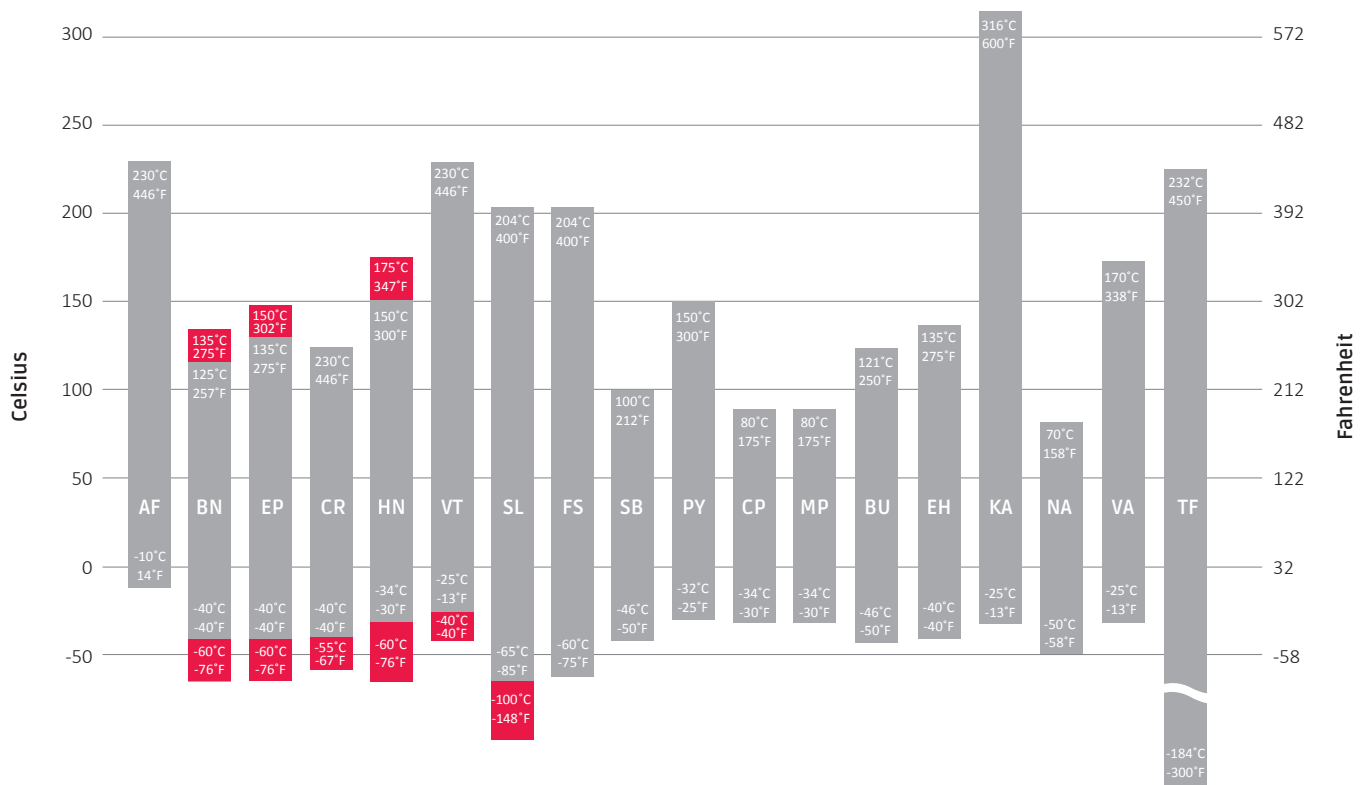
Illustration 5.4, Typical O-Ring Material Working Temperature Ranges
