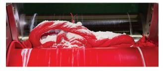
Note: Lubricants can be added directly into rubber compounds to reduce friction. These materials bloom to the surface to add lubricity.
